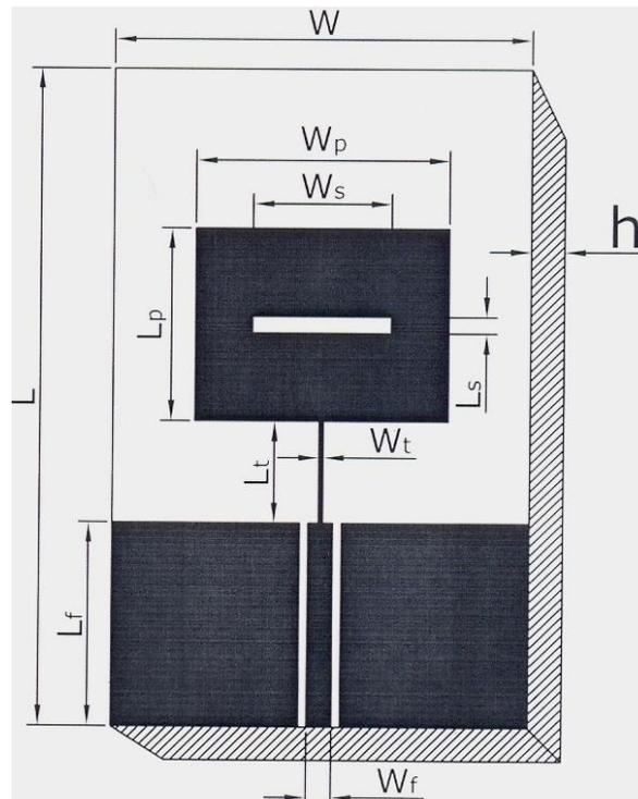
Fig. 1 Top view geometry of SURMSA
