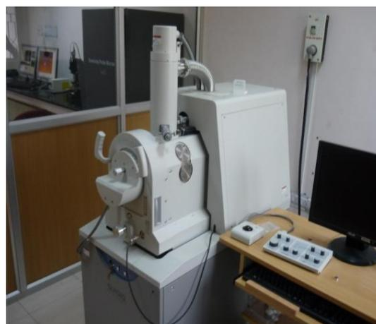
Fig. 2 Hitachi SU- 1510 Scanning Electron Microscope
