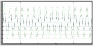
Fig. 6:Output Voltage and Output Current of five level inverter with filter
