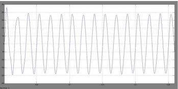
Fig. 5:Output Voltage of five level inverter with filter
