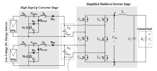
High-Voltage DC Bus Fig. 2 Single-phase multistring five-level inverter topology
