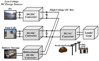
Fig. 1 Configuration of multistring inverter for various DERs application
