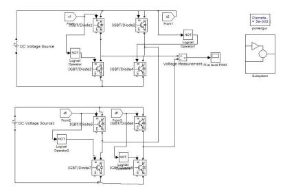
Fig. 3:Simulation diagram of five level inverter
