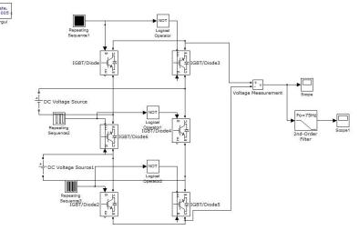
Fig. 7:Simulation diagram of Seven level inverter
