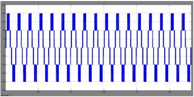
Fig. 6:Output Voltage of five level inverter without filter
