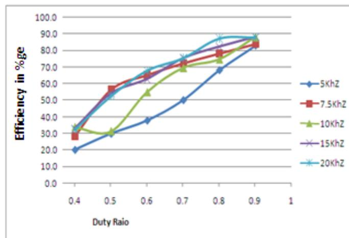
Fig. 13. Efficiency as a function of duty ratio K for different switching frequency.
