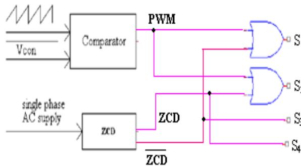
Fig. 3 Block diagram of the control circuit
