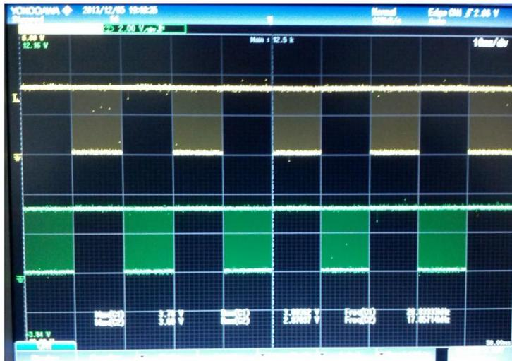
Fig. 7. Gate signal for MOSFETs  $S_1$  and  $S_2$  at  $P=200$  &  $K=0.9$
