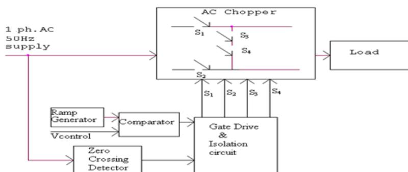
Fig. 1. Block Diagram of the proposed buck AC Chopper
