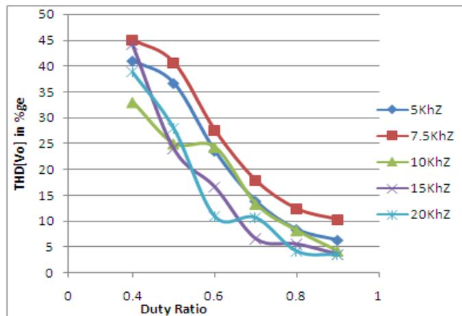
Fig. 12. THD ( $V_o$ ) as a function of duty ratio K for different switching frequency.
