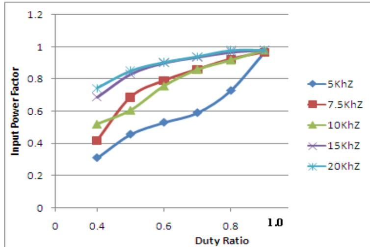
Fig. 10. Input power factor as a function of duty ratio K for different switching frequency.
