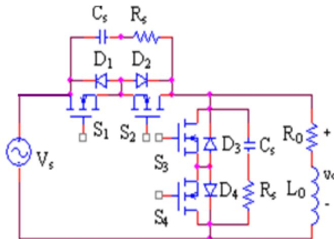
Fig.2. Single-phase Buck AC chopper using bidirectional switches and AC snubbers.
