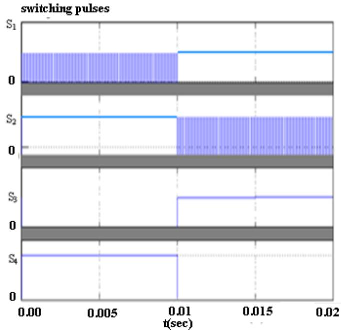
Fig.5. PWM pattern gate control signals.
