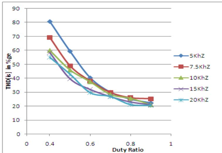
Fig. 11. THD (I<sub>s</sub>) as a function of duty ratio K for different switching frequency.
