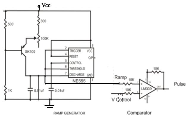
Fig. 4. EPWM pulses generated by comparing ramp with  $V_{control}$
