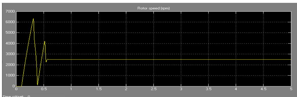
Fig. 7 Simulated speed waveform of BLDC motor in sensorless operation
