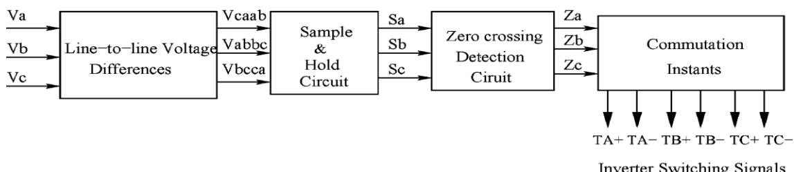
Fig. 2 Functional sequence of operations[8]
