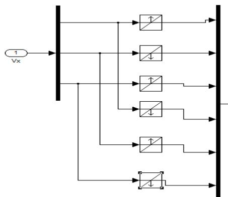
Fig 5 Zero crossing detection model
