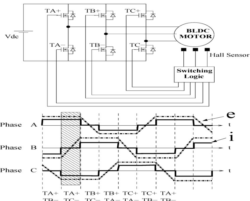
Fig.1. BLDC motor drive along with typical phase current and back EMF[8]
