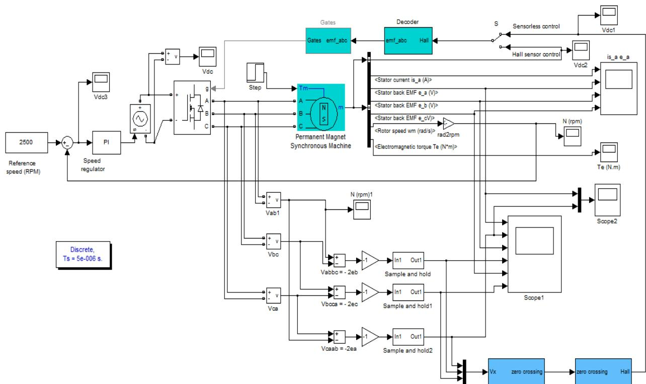
Fig. 3 Simulation of BLDC motor in sensorless mode
