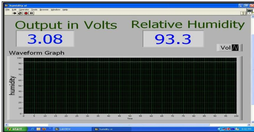
Fig 5: Front panel for humidity measurement
