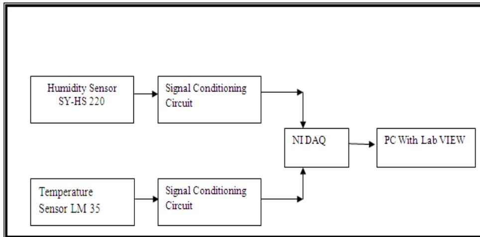
Fig 1: Functional Block Diagram of Humidity and Temperature Measurement System
