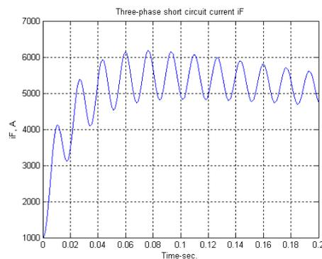
Fig.9: Three-phase short circuit current  $i_c$ . Fig.10: Three-phase short circuit field current  $i_f$
