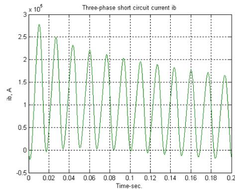
Fig.7: Three-phase short circuit  $i_a$  Fig.8: Three-phase short circuit  $i_b$ .
