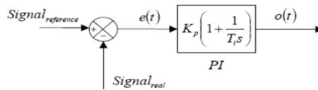
Fig2: General Scheme of PI Controller.
