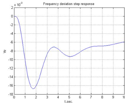
5.b-System output frequency deviation response using PID
