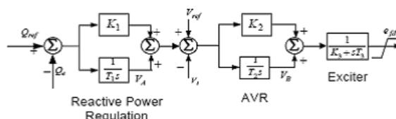
Fig.1: Control block diagram of excitation system.
