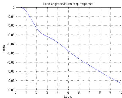
6a-System output load angle deviation response using PI
