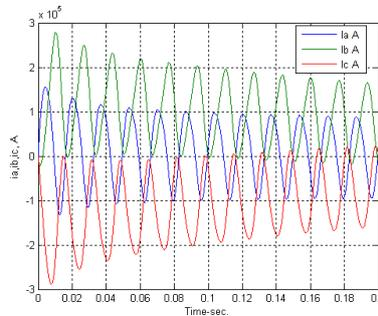
Fig.11: Comparison between three-phases faults  $i_a$ ,  $i_b$  and  $i_c$
