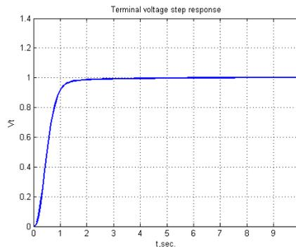
4.b-System output terminal voltage response using PID
