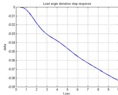
6.b-System output load angle deviation response using PID
