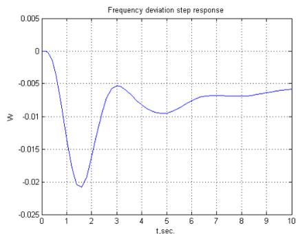
5a.-System output frequency deviation response using PI
