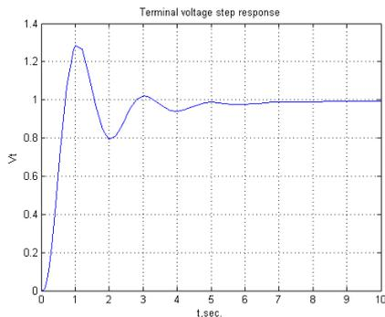
4a-System output terminal voltage response using PI
