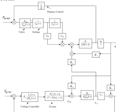
Fig.3: Block diagram of unit including primary and voltage controller.
