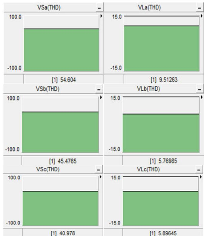
Fig. 9 THD analysis of source voltages and load voltages for three phases
