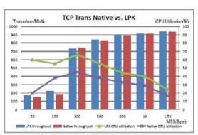
(b) TCP Transmission Fig.6 SATA Performance Vs LPK
