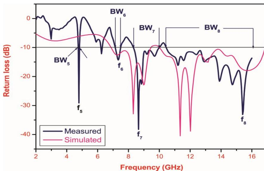
Fig. 4 Variation of return loss versus frequency of MHCMA
