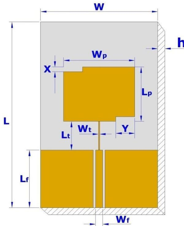
Fig. 1 Top view geometry of TCTURMSA
