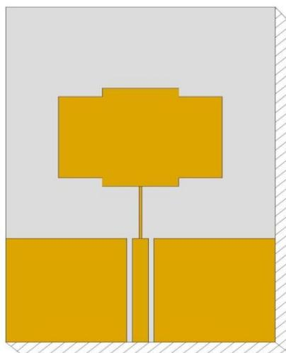
Fig. 2 Top view geometry of FCTURMSA
