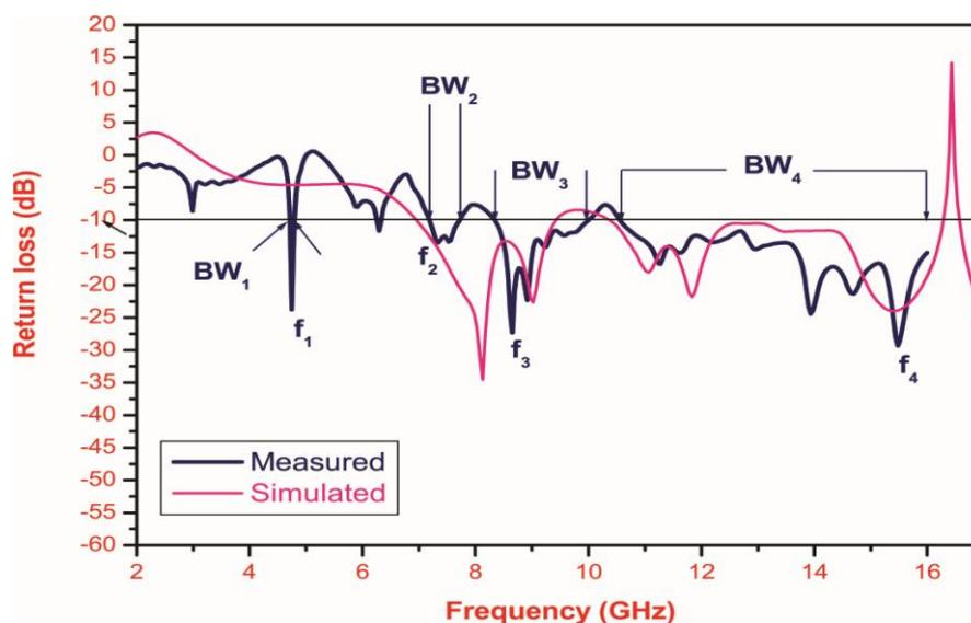
Fig. 3 Variation of return loss versus frequency of TCTURMSA
