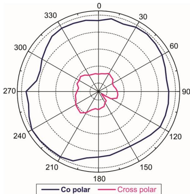
Fig. 6 Typical radiation pattern FCTURMSA measured at 4.76 GHz
