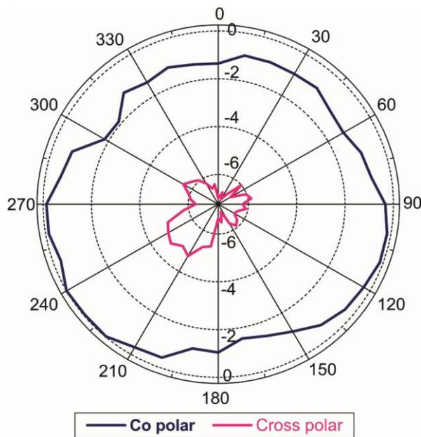
Fig. 5 Typical radiation pattern of TCTURMSA measured at 4.76 GHz
