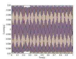
Fig. V Current through the load when batteries are not supporting the Hybrid DSTATCOM.
