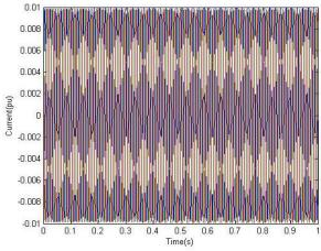
FIG. IX CURRENT THROUGH THE LOAD WHEN BOTH SUPERCAPACITORS AND BATTERIES ARE SUPPORTING THE HYBRID DSTATCOM
