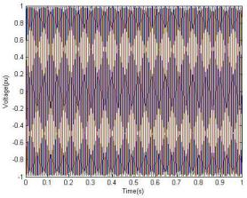
Fig. VIII Voltage across the load when both supercapacitors and batteries are supporting the Hybrid DSTATCOM
