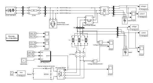
Fig. I Developed Test system for Hybrid DSTATCOM.
