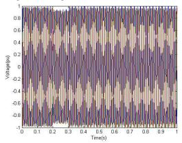
Fig. IV Voltage across the load when batteries are not supporting the Hybrid DSTATCOM.
