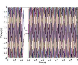
Fig. II Voltage across the load when supercapacitors are not charged
