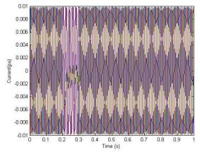
Fig.VII Current through the load when supercapacitors are charged below  $U_{\mbox{\scriptsize min}}$
