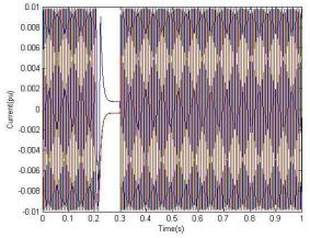
Fig. III Current through the load when supercapacitors are not charged.
