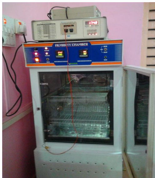
Fig. 6 The experimental arrangement to measure humidity dependant resistance of the composition under investigation
