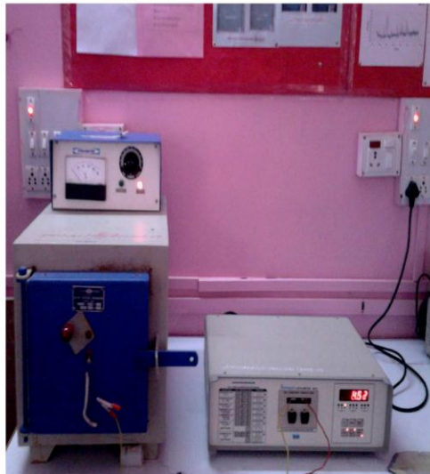
Fig. 4 Experimental set-up to measure temperature dependant resistivity of the composition under investigation
