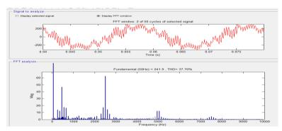
Fig. 9 Harmonic Spectrum of Two level Inverter with filter Phase Voltage at modulation Index=1
