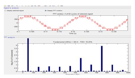
Fig. 18 Harmonic Spectrum of Five level diode clamped Inverter without filter Phase Voltage at modulation Index=1 (PD PWM Technique)
