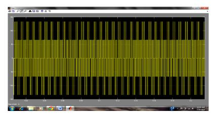
Fig. 11 CMV of Three Level Diode Clamped Inverter(PD PWM Technique) without filter
