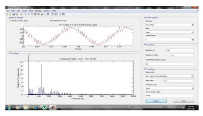
Fig. 15 Harmonic Spectrum of Three level diode clamped Inverter with filter of Phase Voltage at modulation Index=1
