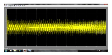
Fig. 20 CMV of Five Level Diode Clamped Inverter(PD PWM Technique) with filter
