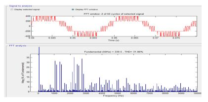
Fig. 12 Harmonic Spectrum of Three level diode clamped Inverter without filter Phase Voltage at modulation Index=1 (PD PWM Technique)
