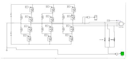
Fig. 10 Model of Three Level Diode Clamped Inverter fed Three Phase Induction Motor without filter
