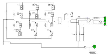
Fig. 13 Model of Three Level Diode Clamped Inverter fed Three Phase Induction Motor with filter
