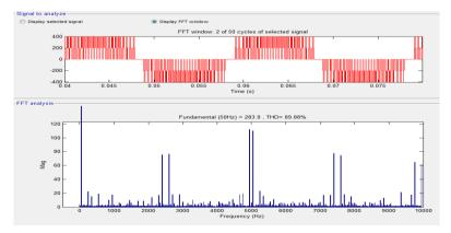
Fig. 6 Harmonic Spectrum of Two level Inverter without filter Phase Voltage at modulation Index=1
