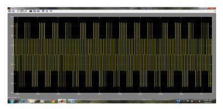
Fig. 17 CMV of Five Level Diode Clamped Inverter(PD PWM Technique) without filter
