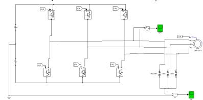
A) Simulation of Two Level Diode Clamped Inverter Induction Motor without filter-
