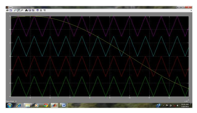
Fig.2 Triangular Waveform Simulation of Five Level Diode Clamped Inverter (PD PWM Technique)
