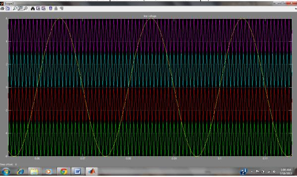
Fig. 9 Sine Waveform Simulation of Five Level Diode Clamped Inverter.(APOD PWM Technique)
