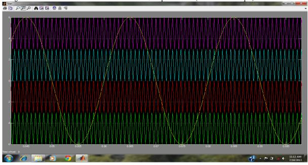
Fig. 1 Sine Waveform Simulation of Five Level Diode Clamped Inverter.(PD PWM Technique)
