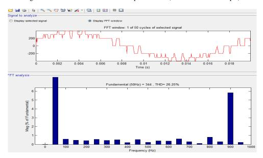
Fig.12 Harmonic Spectrum of Five level diode clamped Inverter Phase Voltage at modulation Index=1 (APOD PWM Technique).
