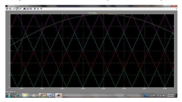
Fig 10 Triangular Waveform Simulation of Five Level Diode Clamped Inverter (APOD PWM Technique)
