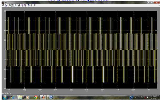
Fig. 3 CMV of Five Level Diode Clamped Inverter(PD PWM Technique)
