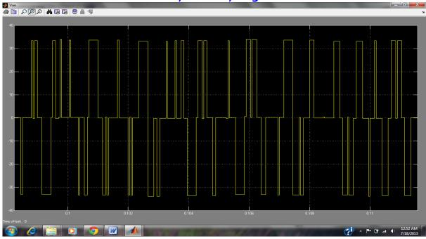
Fig.7 CMV of Five Level Diode Clamped Inverter(POD PWM Technique)
