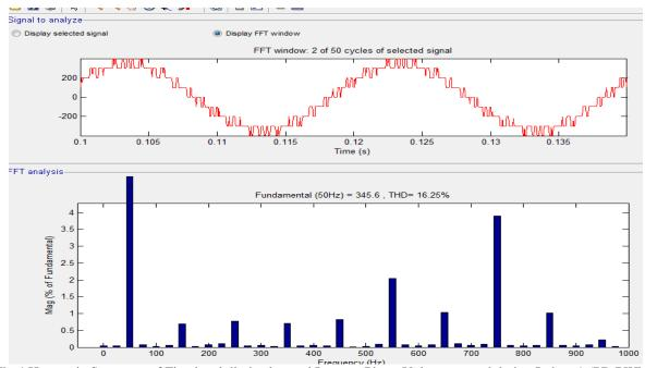
Fig.4 Harmonic Spectrum of Five level diode clamped Inverter Phase Voltage at modulation Index=1 (PD PWM Technique)
