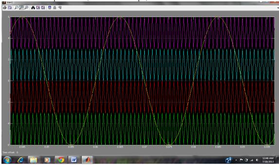
Fig.5 Sine Waveform Simulation of Five Level Diode Clamped Inverter.(POD PWM Technique)
