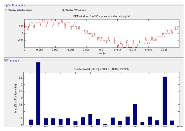
Fig.8 Harmonic Spectrum of Five level diode clamped Inverter Phase Voltage at modulation Index=1 (POD PWM Technique)
