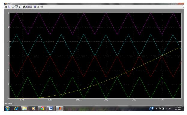
Fig.6 Triangular Waveform Simulation of Five Level Diode Clamped Inverter (POD PWM Technique)
