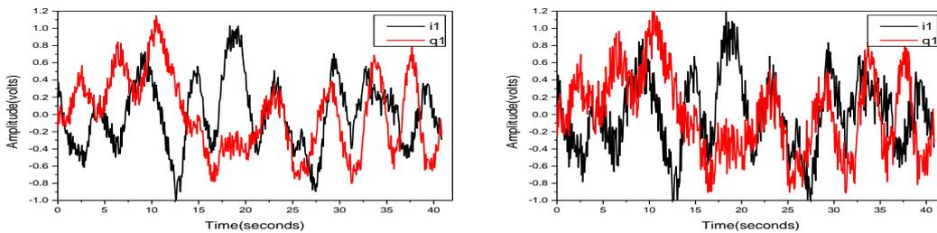
Fig. 6 Real and imaginary components of model-produced time series using the VHF simulation Parameters for first receiver with added noise level of 20% and 40%.
