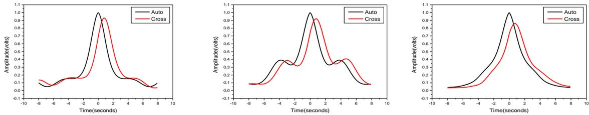
Fig. 4 Auto and Cross correlation function for the receiver pair 1-3 with turbulent RMS velocity of 10%, 15% and 20% respectively of steady state wind vector.
