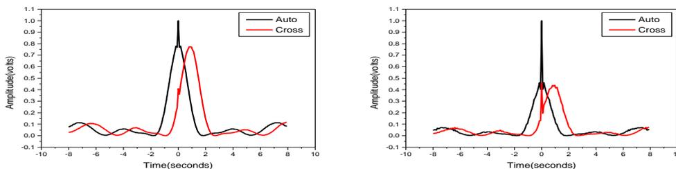
Fig. 7 Auto and cross correlation function for the Rx pair 1-3 with noise level of 20% and 40% respectively.
