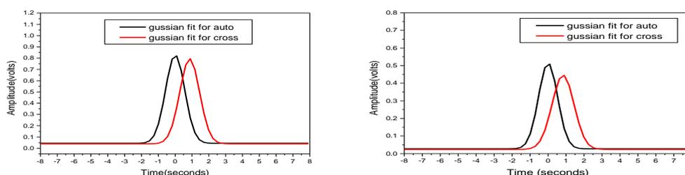
Fig. 8 Least squares Gaussian fit for the auto and cross correlation function for the Rx pair 1-3 with noise level of 20% and 40% respectively
