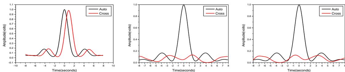
Fig. 3 Auto and cross correlation function for the Rx pair 1-3, 1-2, 2-3 respectively.
