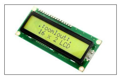
Fig 5.2 LCD 16x2 (Liquid-Crystal Display)
