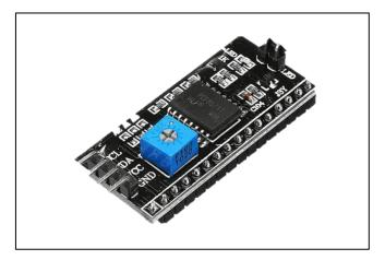
Fig 5.2 I2C (Inter-Intergrated Circuit)
