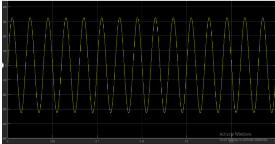
Fig:9 Output Voltage of Inverter
