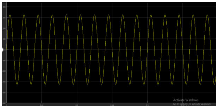
Fig:5 Output Voltage of inverter
