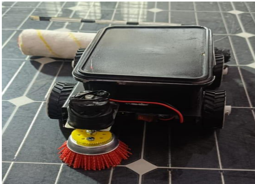
Fig 2 solar panel cleaning robot on the solar panel
