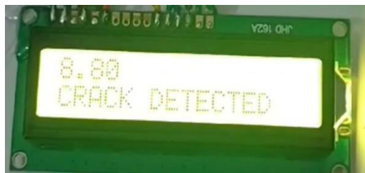
Fig. 13 Display showing crack detected by ultrasonic sensor including its depth
