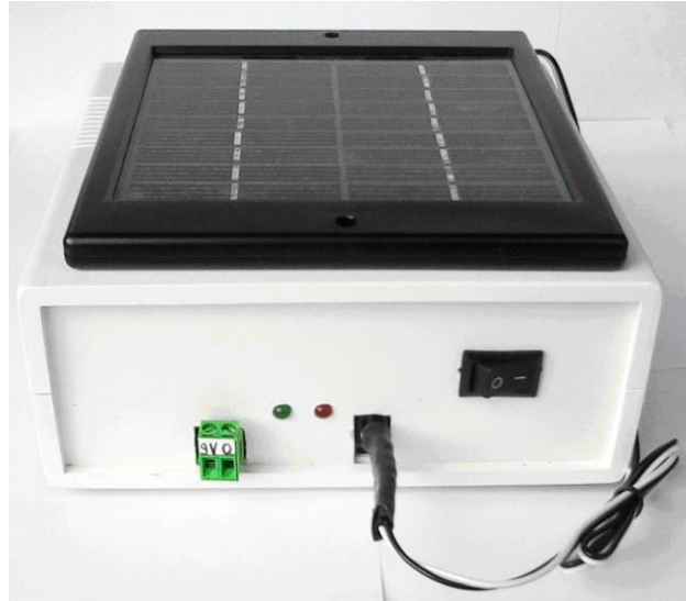
Fig. 2 Front view of the device for battery charging of the mobile phone
