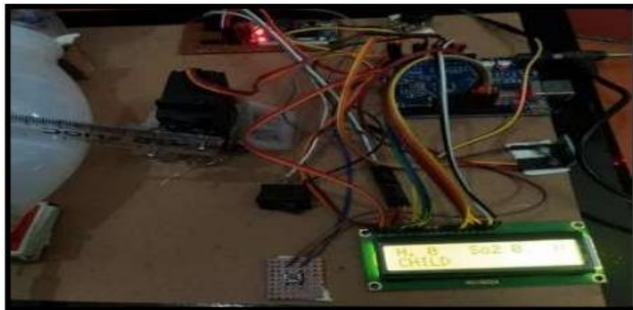
Figure 2: Child Mode, In this mode the frequency of pumping is adjusted in accordance with the physical requirements of a child.
