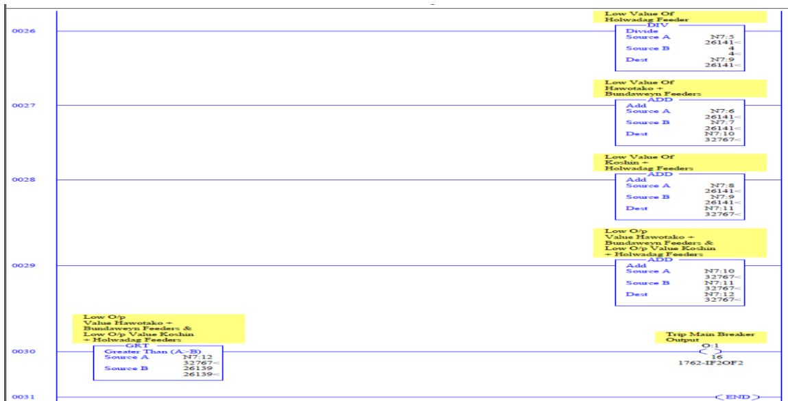
Figure 0.2 Adding of low values of every feeder Current
