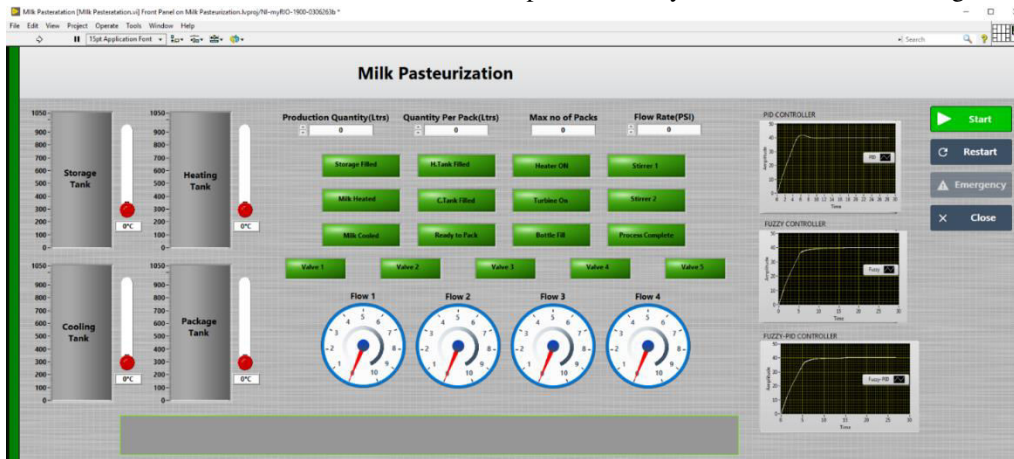
Fig. 8. Response of PID controller, fuzzy controller and fuzzy-PID controller in Front Panel
