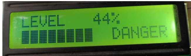
Fig 7: When gas leakage reaches the threshold level
