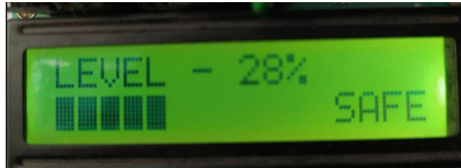
Fig 6: Gas leakage below threshold level
