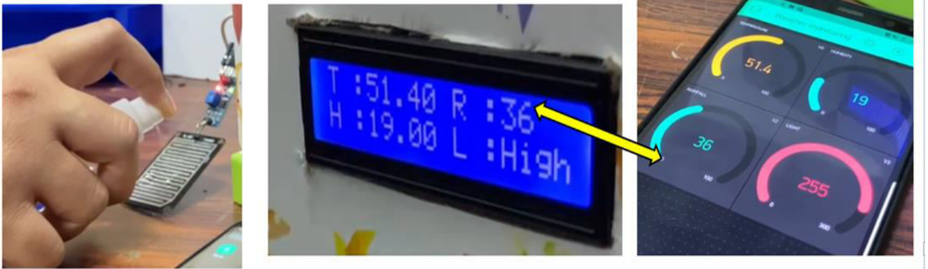
Fig. 8 Testing of Rain level sensor
