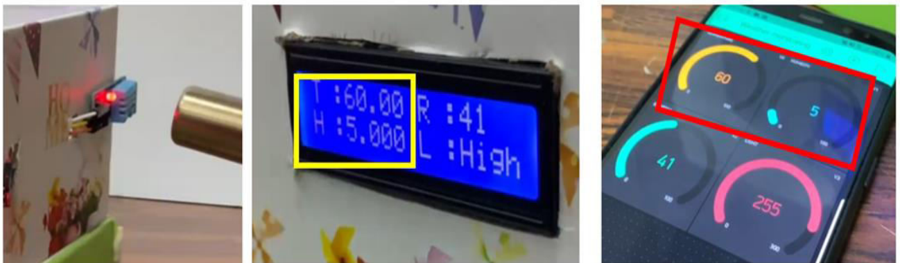
Fig. 9 Testing of Temperature and humidity sensor
