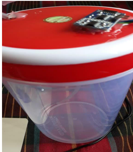
Figure 5: Water Tank with Ultra Sonic Sensor
