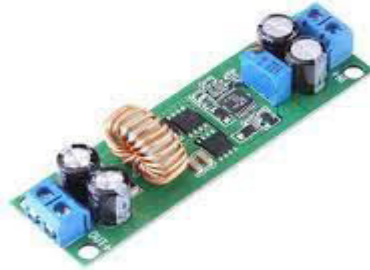
Fig.3: Dc to Dc Convertor.
