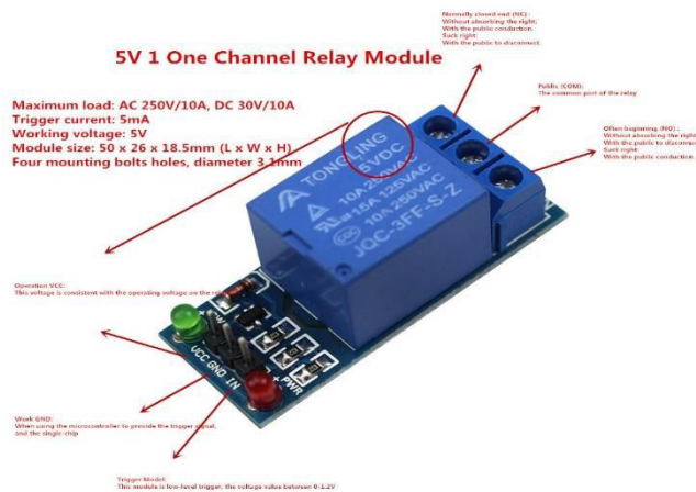
Fig 2:Single-Channel Relay Module Specifications
