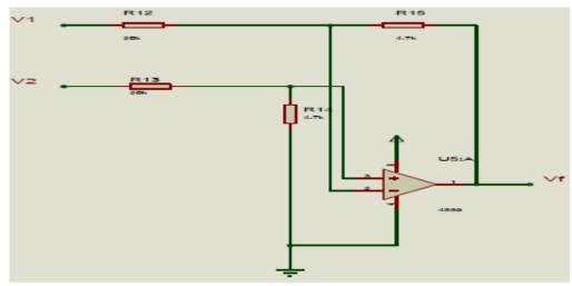
Figure 7: Output feedback circuit
