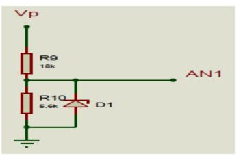
Figure 8: Voltage sensing circuit
