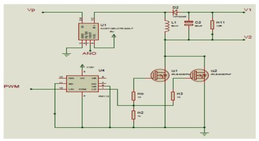
Figure 6: Circuit diagram of a Buck-Boost Converter (Driver unit)
