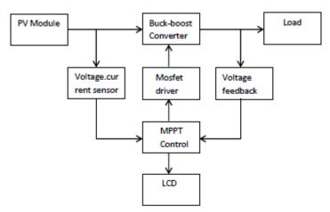
Figure 1: Block diagram of solar PV System [8]
