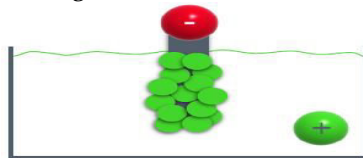
Fig. 9. Cathode when Electrical voltage is applied The base coat is attracted by the metallic surface.
