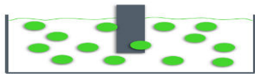
Fig. 8. Cathode when No voltage applied The base coat is not attracted by the metallic surface
