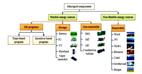
Figure 1: Microgrid Component
