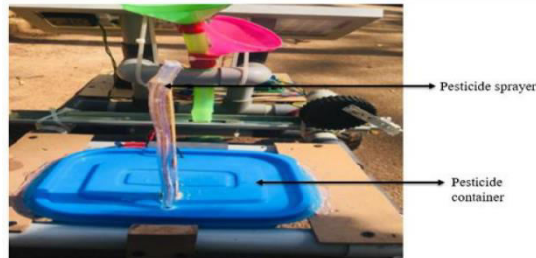
Fig.13 Snapshot of seed pesticide spraying mechanism
