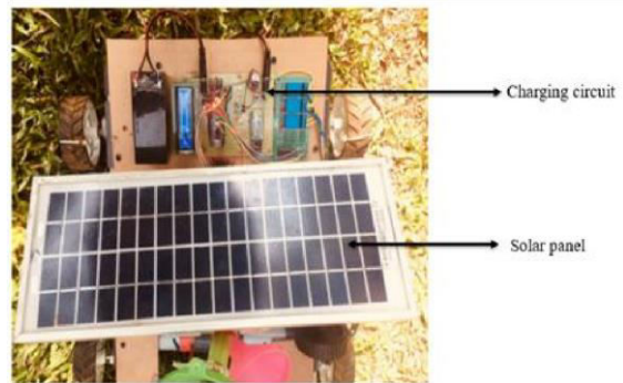
Fig.10 Snapshot of solar charging.
