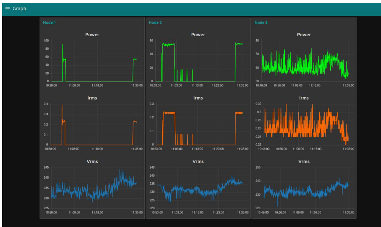
Fig.6. Graphical analysis of real time data of voltage , current and power consumption .
