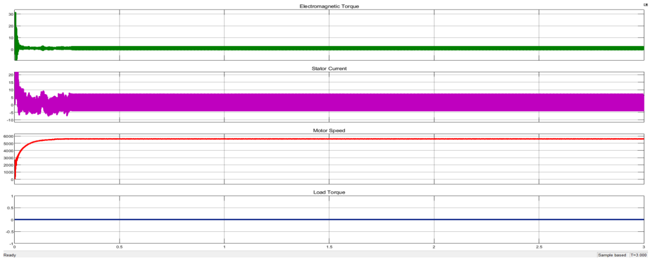
Fig. 15 Torque, stator current, Speed waveform of NIBFE-VSI-BLDC motor system
