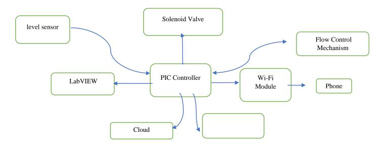
Once the module Starts first patient details (i.e.) Body temperature is measured by sensor. These details are stored in server by LabVIEW and after that solenoid valve (1) getting energized by PIC Controller and tripping will starts.
