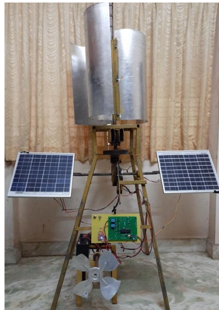
Figure. 5 Prototype of the Solar and Wind Hybrid Marine Propulsion System
