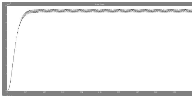
Fig 6. Power output with normal gating pulse
