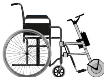
Fig. 1 Motorized and detachable driving module with a generic manual wheelchair
