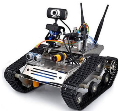
Surveillance robot mounted on metal tracks
