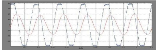
**Fig 11. Link current and scaled voltage in the improved ac-link buck–boost inverter (simulation, dc– ac power flow).**
