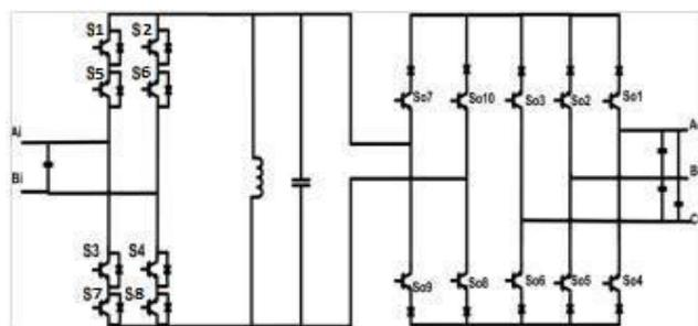
Fig.4. Improved AC-link buck-boost inverter with reverse-blocking IGBTs.
