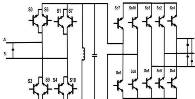
Fig 3. Proposed eighteen switch improved ac-link buck– boost inverter.
