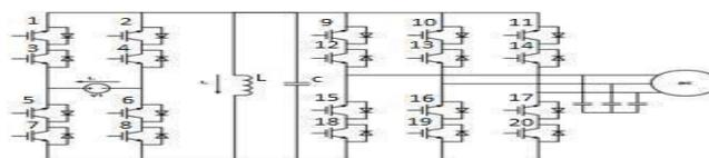
Fig. 1. Conventional AC-link buck–boost inverter
