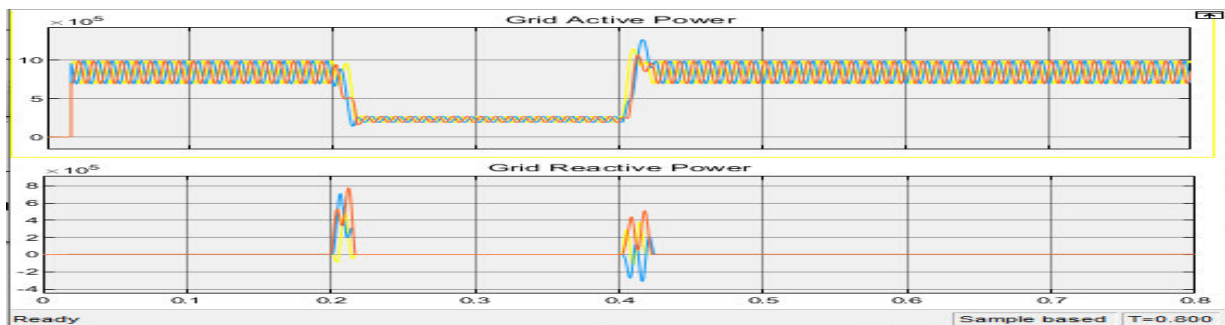
Figure 4.3: Grid Active and Reactive Power Response Before and After Fault with STATCOM Support
