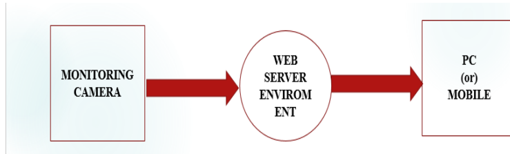
Fig.No.2 Block diagram of camera monitoring system
