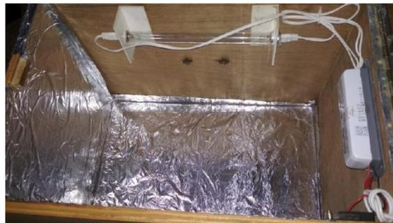
Fig.3 Inner view of UV sterilization box
