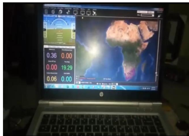
Fig 5. Configuration of Flight controller using Mission planner
