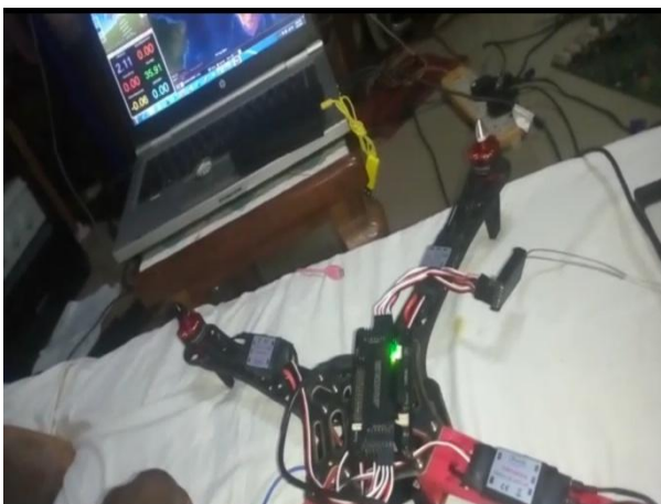
Fig 5. Configuration of Flight controller using Mission planner
