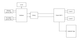
Fig 1 block diagram of partial load shedding management system
