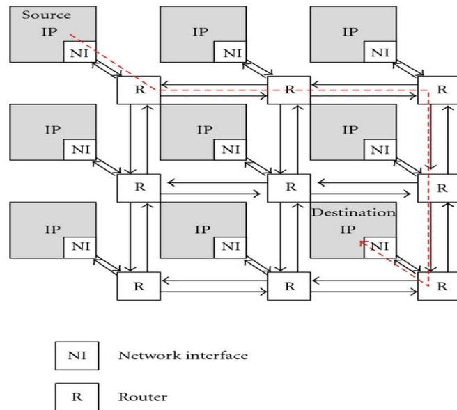
Figure 1: Typical NoC structure in a mesh topology
