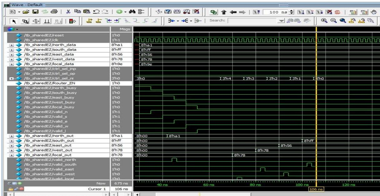
Figure 4: Simulation Waveforms of Proposed EZ Pass Router
