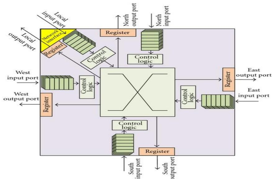
Figure 2: Typical NoC router architecture
