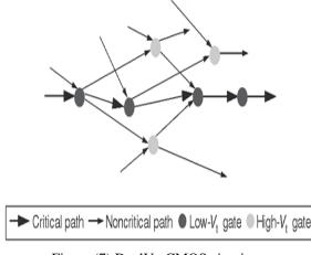
Figure (7) DualV<sub>th</sub> CMOS circuitry.
