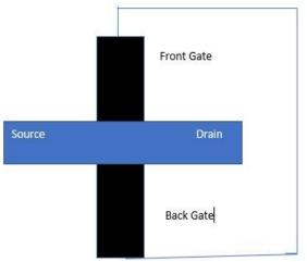
Figure(8)Structure of DGDT-SOI MOSFET.
