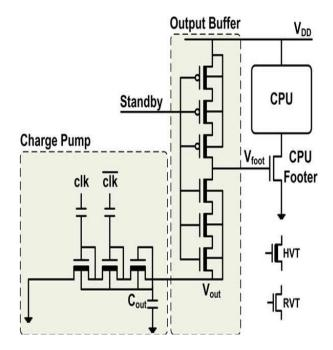
Figure (13) Reducing standby leakage current for power gated blocks.
