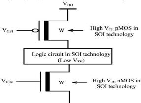
Figure (4) MTCMOS circuitry. The working of MTCMOS can be explained asunder:
