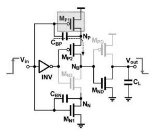
Figure15 (b) Proposed Bootstrap Circuit showing transition from low to high.
