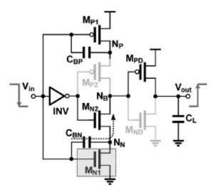
Figure15 (a) Proposed Bootstrap Circuit showing transition from high to low.
