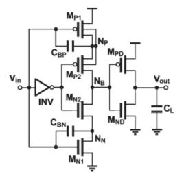
Fig(15) Proposed Bootstrap circuit.
