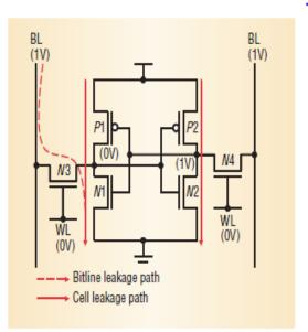
Figure (10) leakage currents and their paths in memory
