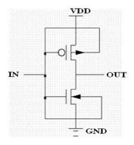
Figure (6) Schematic of DTCMOS inverter
