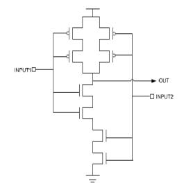
Figure (14) Stack effect in of 2 I/P NAND gate.
