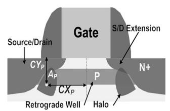
Figure (11) Nano scaled N channel device with super steep retrograde and halo doping.
