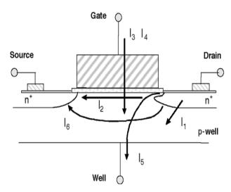
Figure (3) describe six short channel leakages [2].
