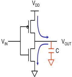
Figure 1 Leakage Power Dissipation.
