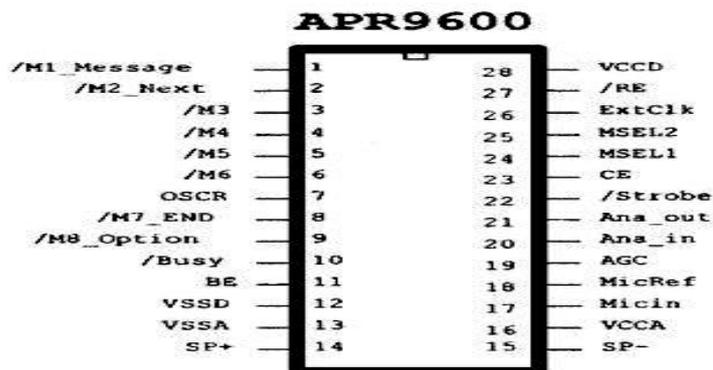
Fig 14:APR Pin diagram
