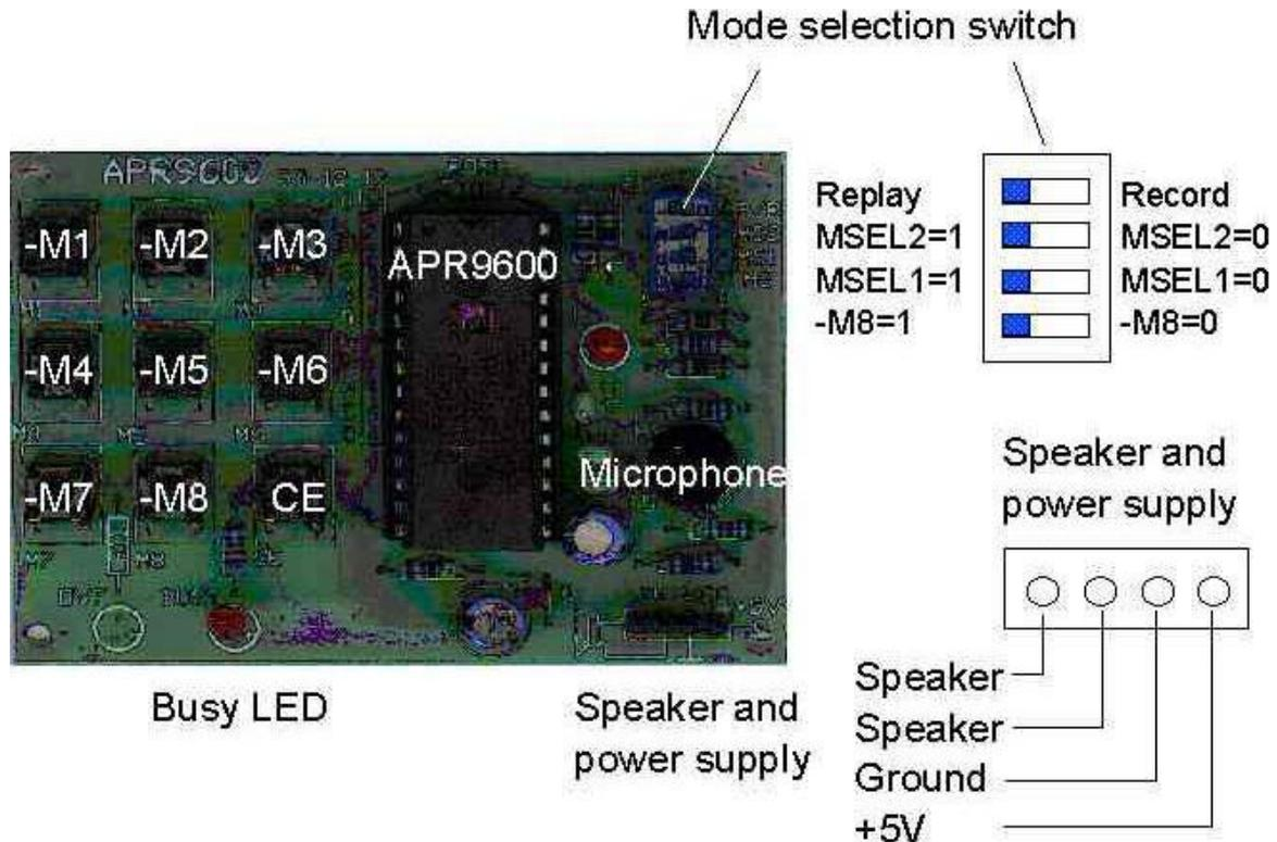
**Fig 15: APR9600 module with connector details (to record in parallel mode, the switch setting should be same as displayed above. To record, the top switch should be on the right-hand side. To replay, the top switch should be on the left.**
