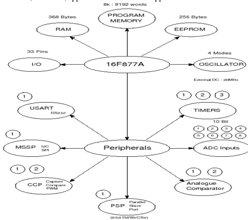
**Fig2:Peripherals of PIC microcontroller**
