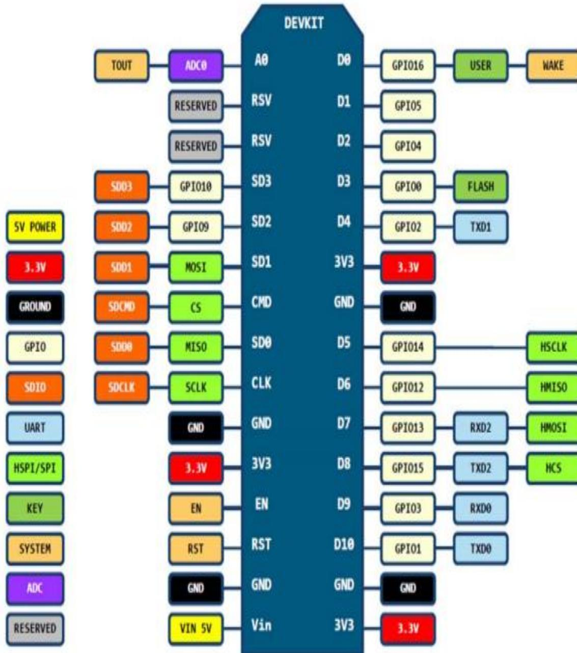
Fig 9:NODEMCU Pin configuration
