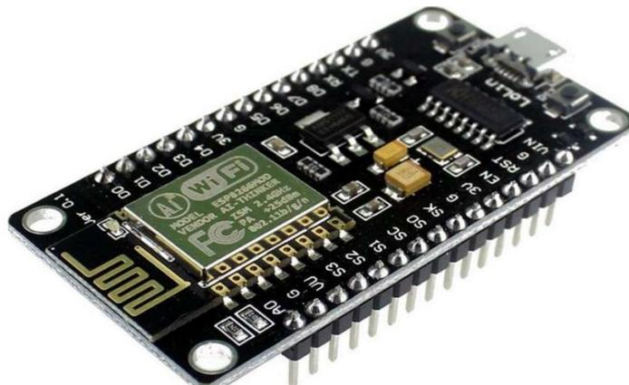
Fig 7: ESP-12E BASED NODEMCU
