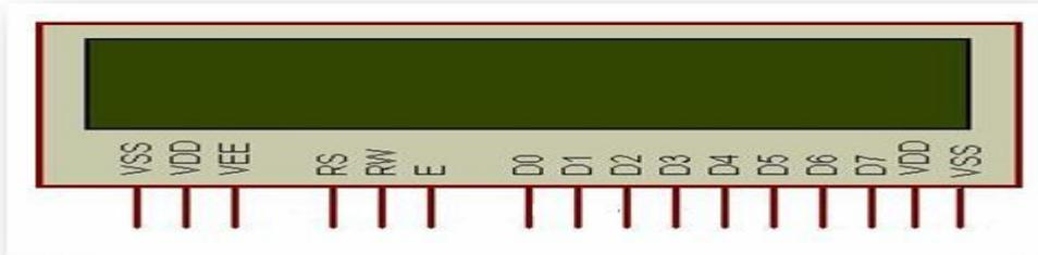
Fig 12:Pin diagram of LCD
