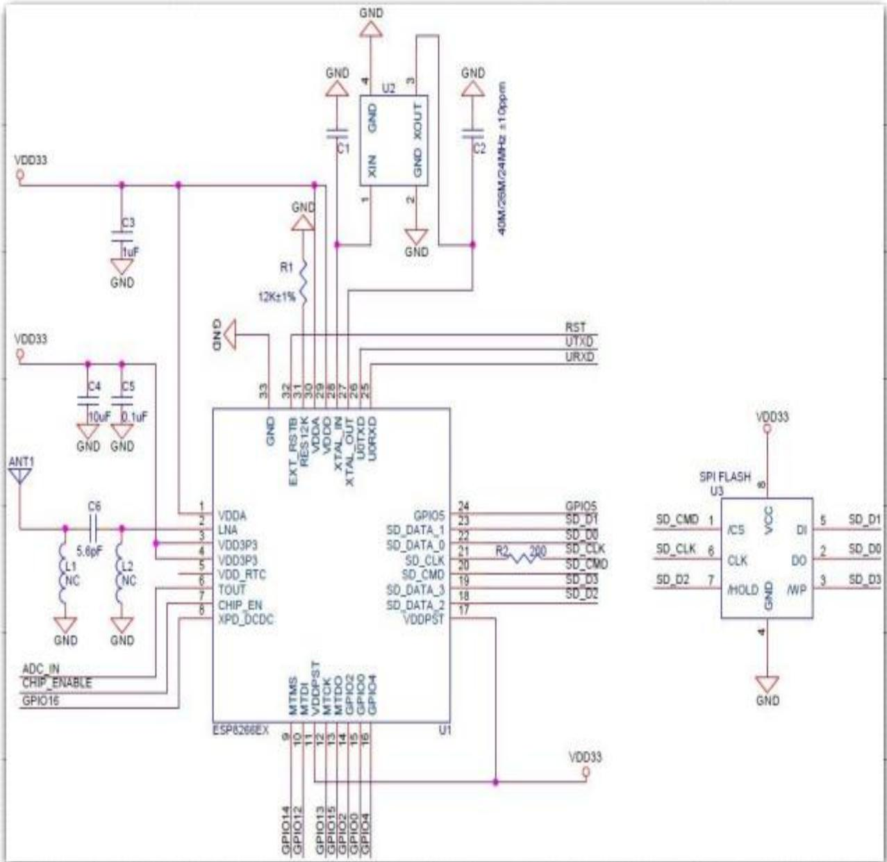
Fig 10: Schematic diagram of WIFI module
