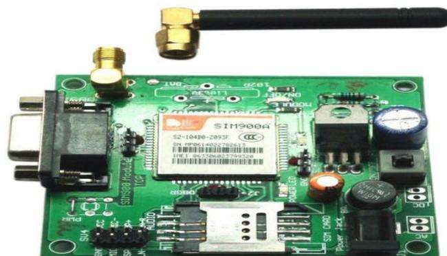
**Fig 5: GSM modem**
