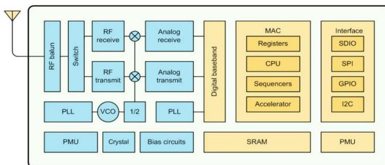
Fig 8: Integrated SOC of NODE MCU
