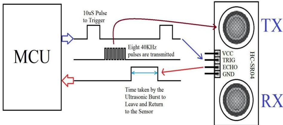
**Fig 4: Working of ultrasonic sensor**
