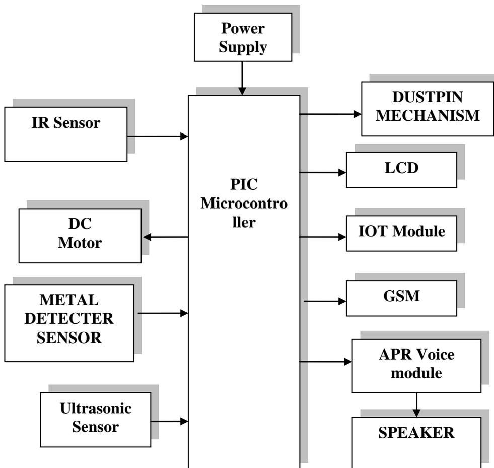
Fig 17 :block diagram of proposed system
