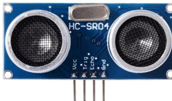
**Fig 3:Ultrasonic sensor**
