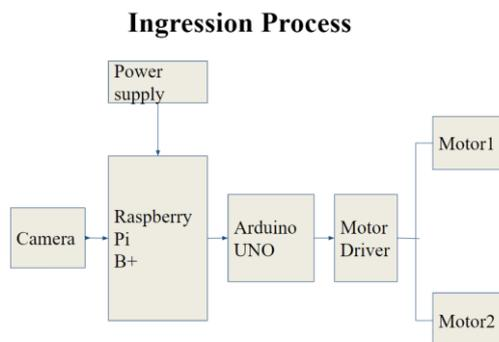
Fig 2) Block diagram of Ingression Process
