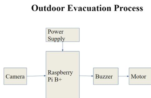
Fig3)Block diagram of Evacuation Process
