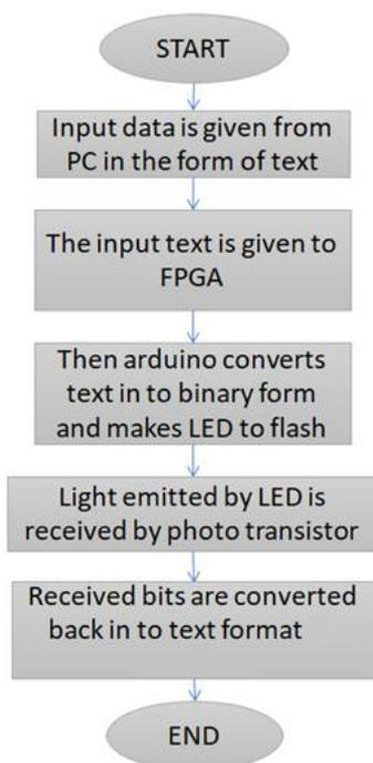
Fig.1 Proposed System Flow Diagram
