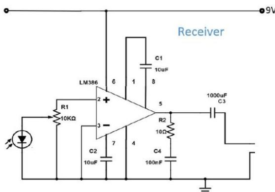
Fig.3 Proposed System Receiver Circuit
